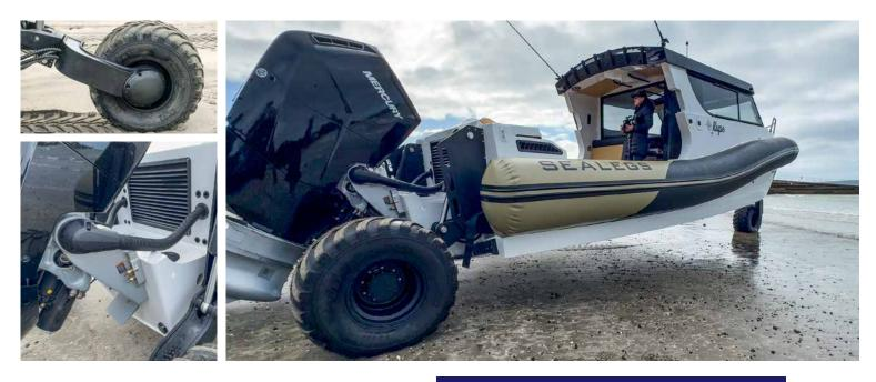
position. Kupe doesn't have a boarding ladder, so this ability to squat makes it easier to scramble on over the wheels at the transom, utilising the well-positioned hand-holds. (There is also an option of an electrically driven swim platform which extends out the side of the hull, but that box didn't get ticked, to save weight.) This 'squat' function also makes it easy to drain any water out of the bilge.
