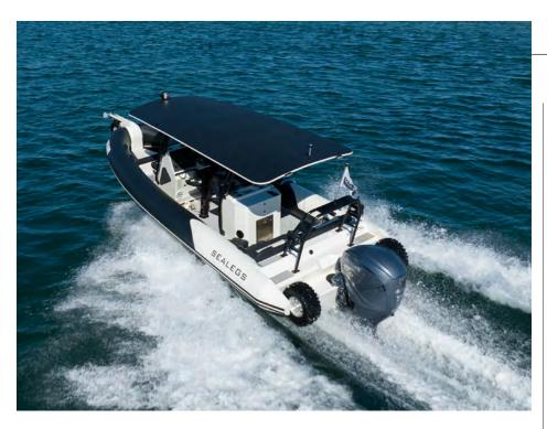
All Sealegs amphibious crafts come with All Wheel Drive (AWD) and Seastar power-assisted hydraulic steering with EPS. Both the front wheel and rear wheels have their own wheel motor that allows for maximum traction and terrain capability.
