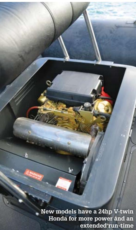
**New models have a 24hp V-twin Honda for more power and an extended run-time**
